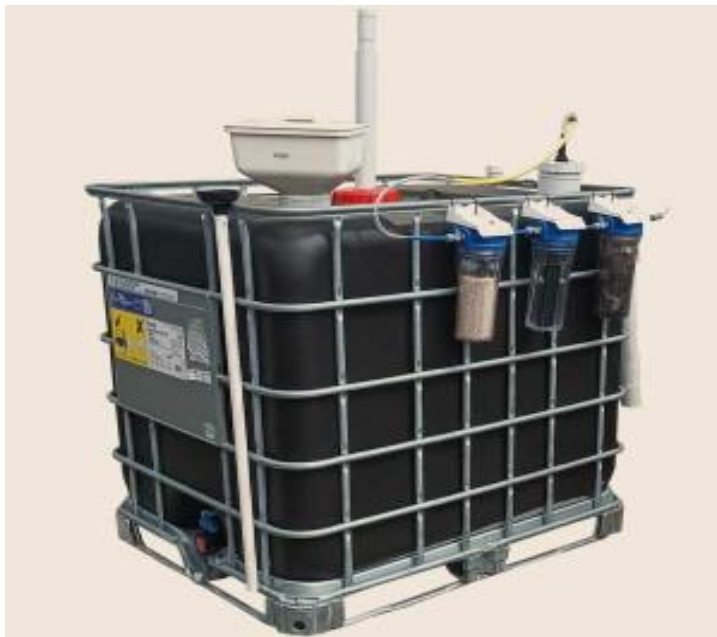
Figure 1 : Example of a 1000 L IBC reactor tank
