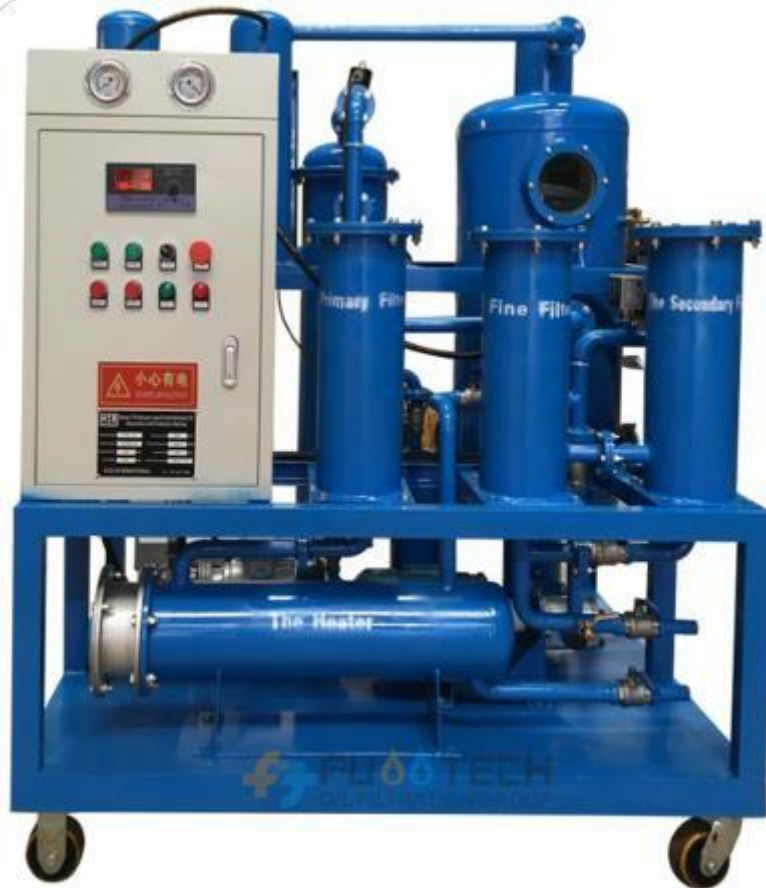
Figure 2: Typical mobile oil purifier photo
