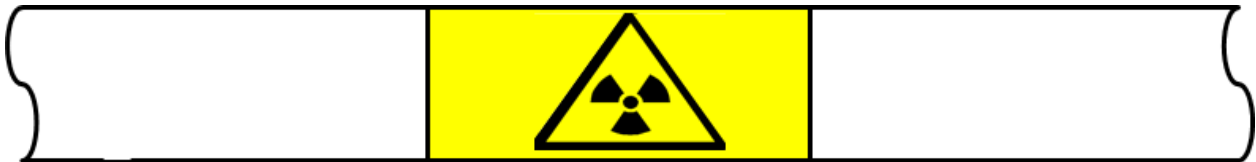
Figure 20: Ionizing Radiation Hazard Symbol with Golden Yellow Band
