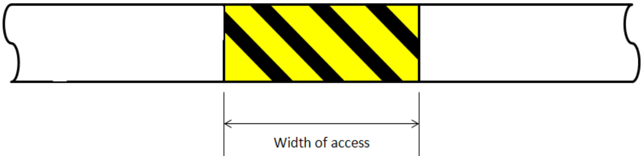
Figure 18: Golden Yellow Bands with Superimposed Black Diagonal Strips
