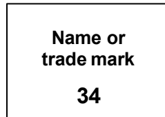
Figure 15 – Label to include the size (size label may not be a separate label)
