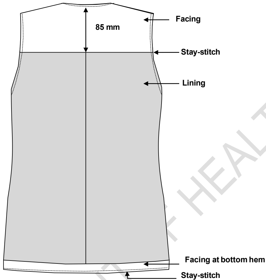
Figure 8 – Back lining and facings (inside view)
