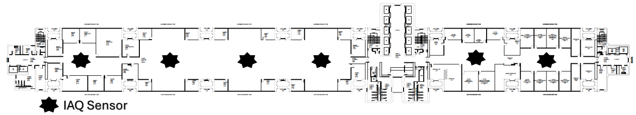
Figure 11: Tower Building proposed sensor positioning 14 th floor (6)
