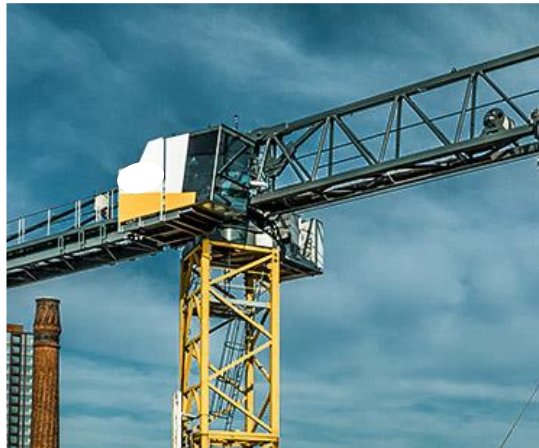
Flat Top Tower Crane
