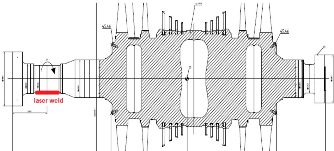
Figure 1: Typical LP Rotor (laser weld journal as indicated in red)
