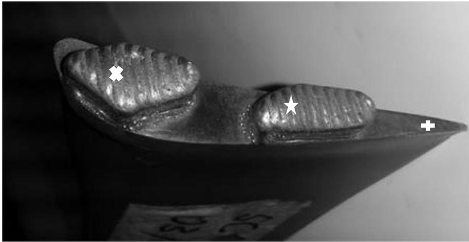
Figure 3: Required thermocouple positions for the tenon PWHT cycle
