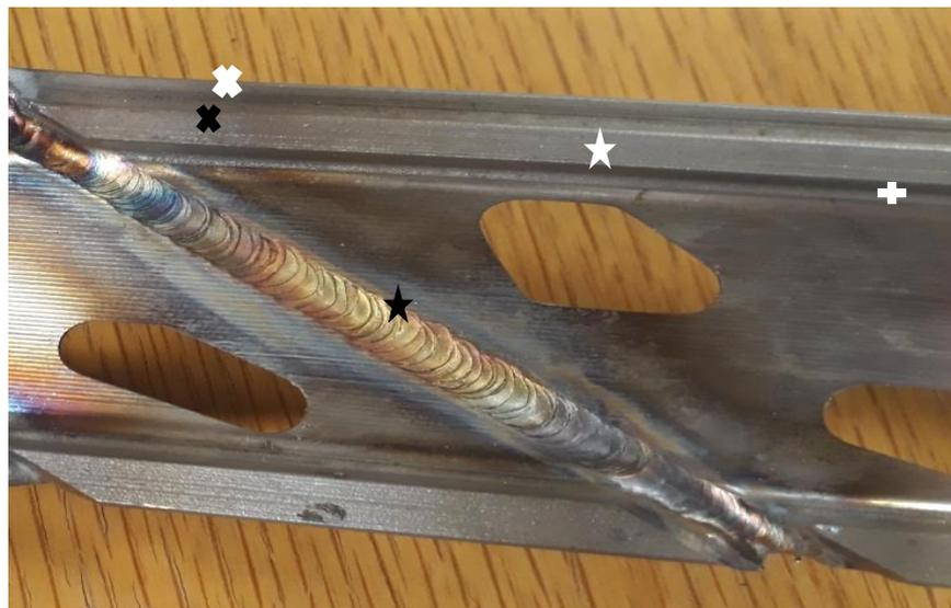
Figure 5: Required thermocouple positions for the shroud PWHT cycle
