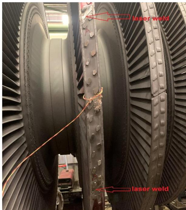
Figure 4: Illustration of laser welding on shroud
