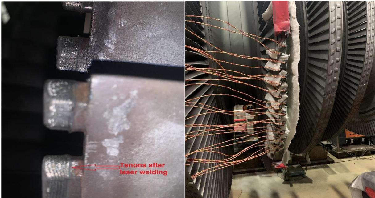
Figure 2: (a). Illustration of Tenons after laser welding, (b). Illustration PWHT set-up
