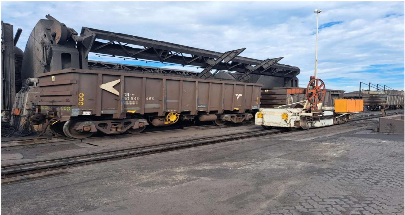
*Figure 1: Charger positioning the wagon*
