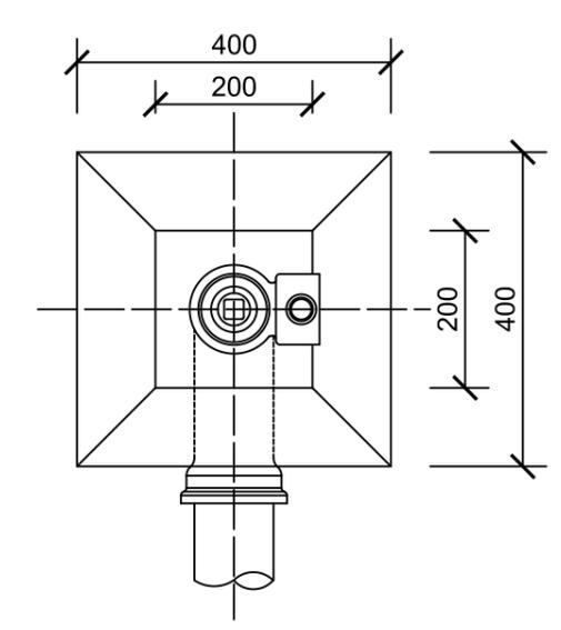
TOP VIEW - TYPE B CONCRETE ANCHOR
