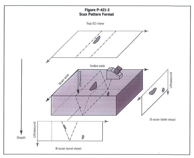
Figure 4: Volume-corrected B-scan, C-scan and D-scan displays
