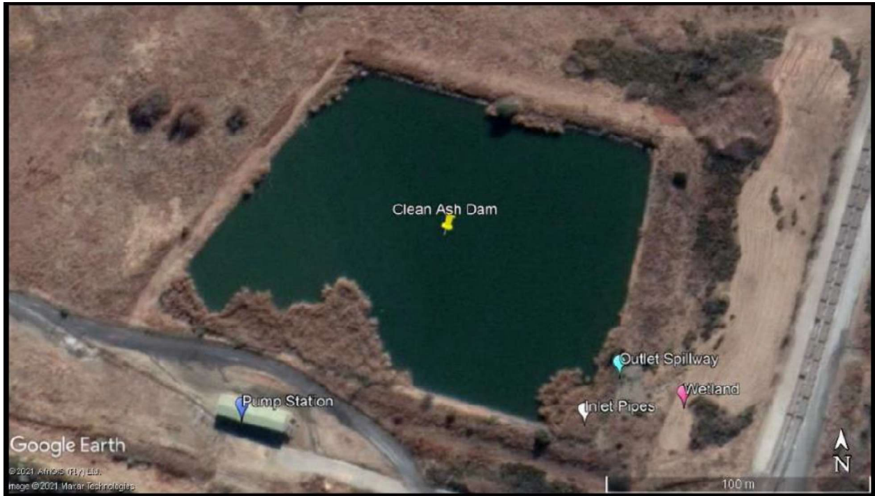
Figure 7: Layout Clean Water Ash Dam
