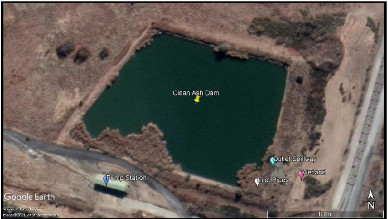
Figure 7: Layout Clean Water Ash Dam
