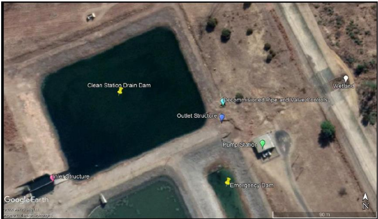
Figure 3: Layout Clean Station Drain Dam
