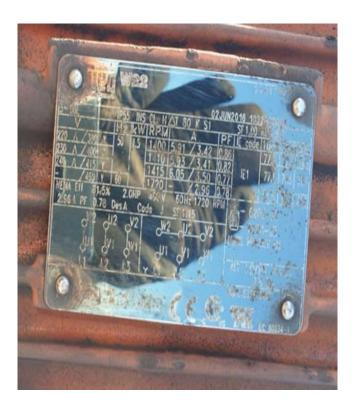
Figure 2: Motor plate
