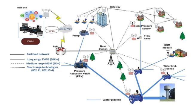
In a Smart Water Network Management (SWNM) the Dynamic Hydraulic Model (DHM) performs forecasting and intelligently control the water flow and introduce a smart pressure control management through the actuation of either a smart pump and/or pressure regulating valves (PRVs). The CSIR have already developed the following:
