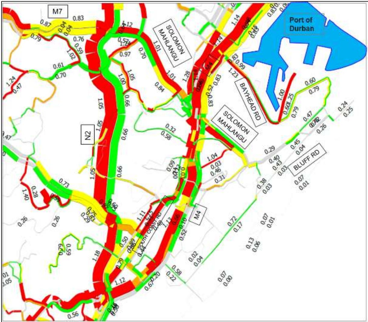
Figure 23: 2035 Level of Service (LOS) network assessment (EMME4 output)
