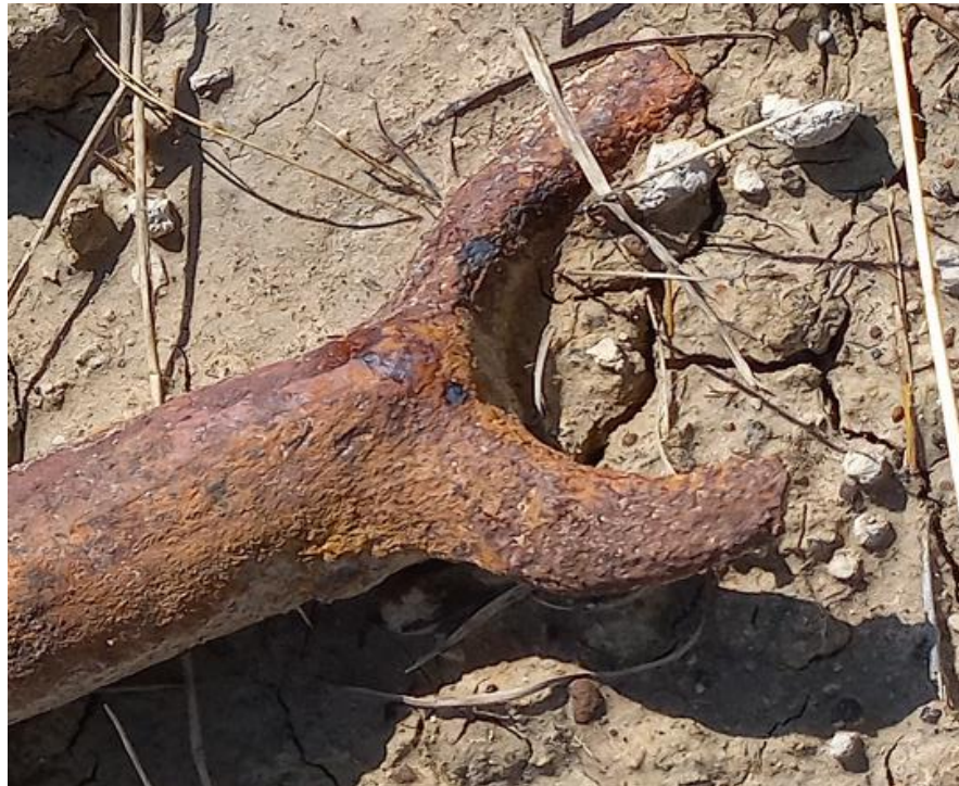
Figure 5: Corroded eye link
