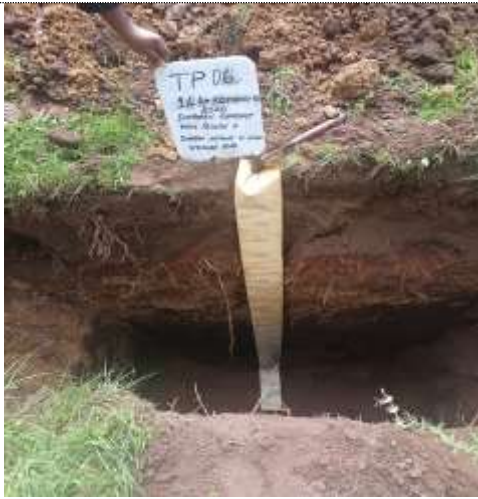
Photo 4: Excavated Trial Pit on site
