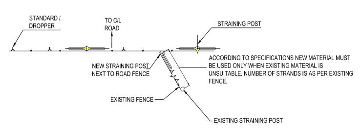
FENCING IN RELATION TO ROAD AND REPAIR OF EXISTING FENCE IF CUT BY ROAD RESERVE SCALE 1:100
