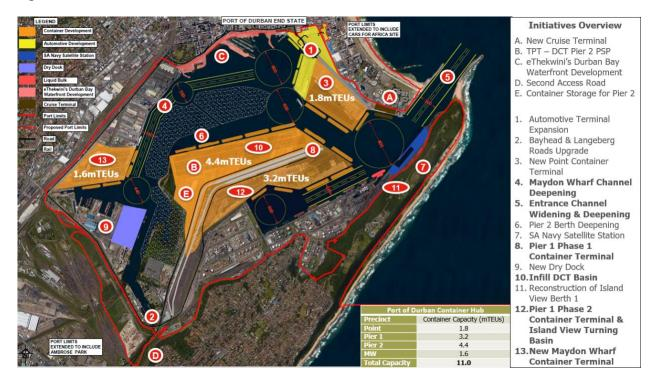
The scope of this pre-feasibility study shall solely focus on Entrance Channel Widening and Deepening, Navigational Studies, Pier 1 Container Terminal Phase 1 & 2, Infill DCT Basin, and Terminal Layout for the New Maydon Wharf container Terminal.
