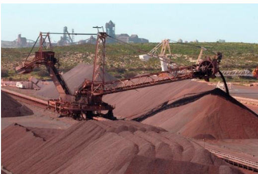
Figure 2. Stacker-reclaimer at BTS
