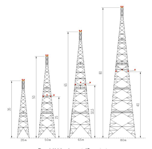
Figure 1: Lighting placement of Tower structures
