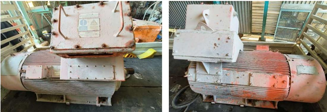
The 360kW motors are used in the Tailings section and Extension 8. They are used at TTPS on line 1 to line 4 and Tailings extension 8 stream A & B. Most of the motors that we still using we installed in 1980's, Due to aging of these motors we are experiencing breakdowns on motor failures. The motors be need to replace after the motor's repair cost has been deemed uneconomical by service provider.
