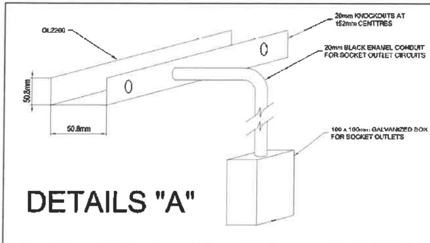
The detail for the installation of the roof and desk consoles is given in the picture below.
