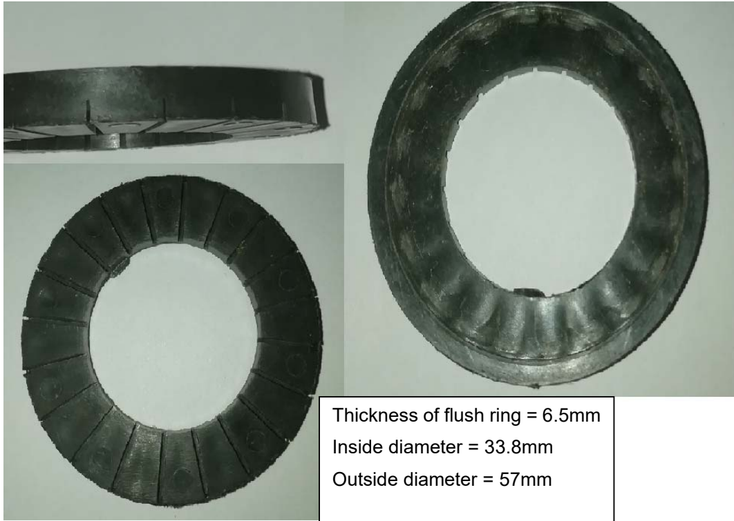
Figure 7: The mixed bed flush ring
