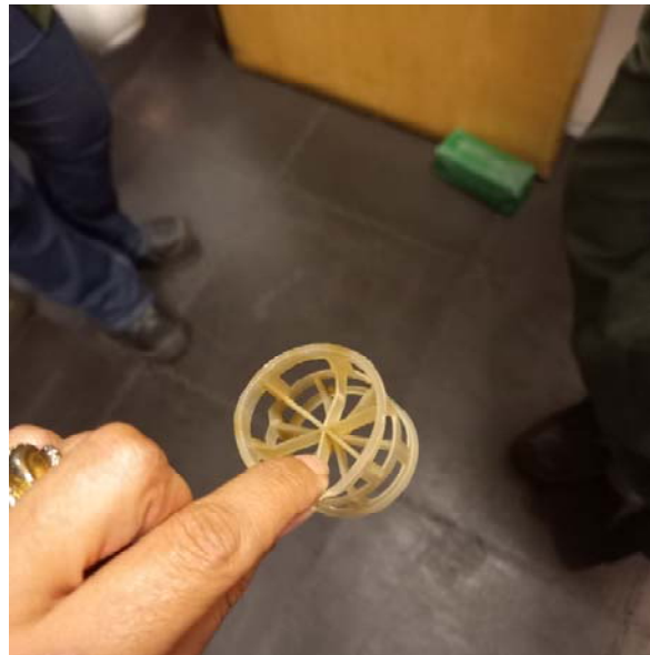
Figure 3: Photo of the pall ring in the degasser
