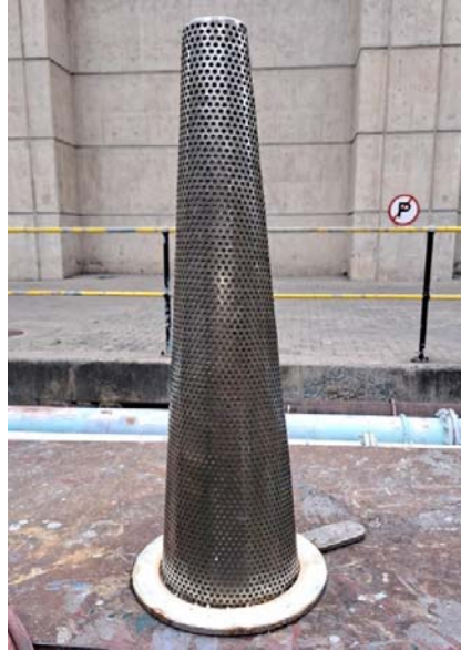
Figure 1: Typical bottom outlet SS316L with hat strainer
