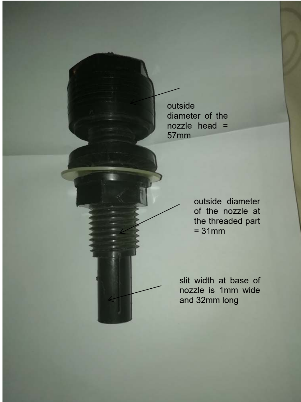
Figure 5: Side view of mixed bed nozzle showing slit
