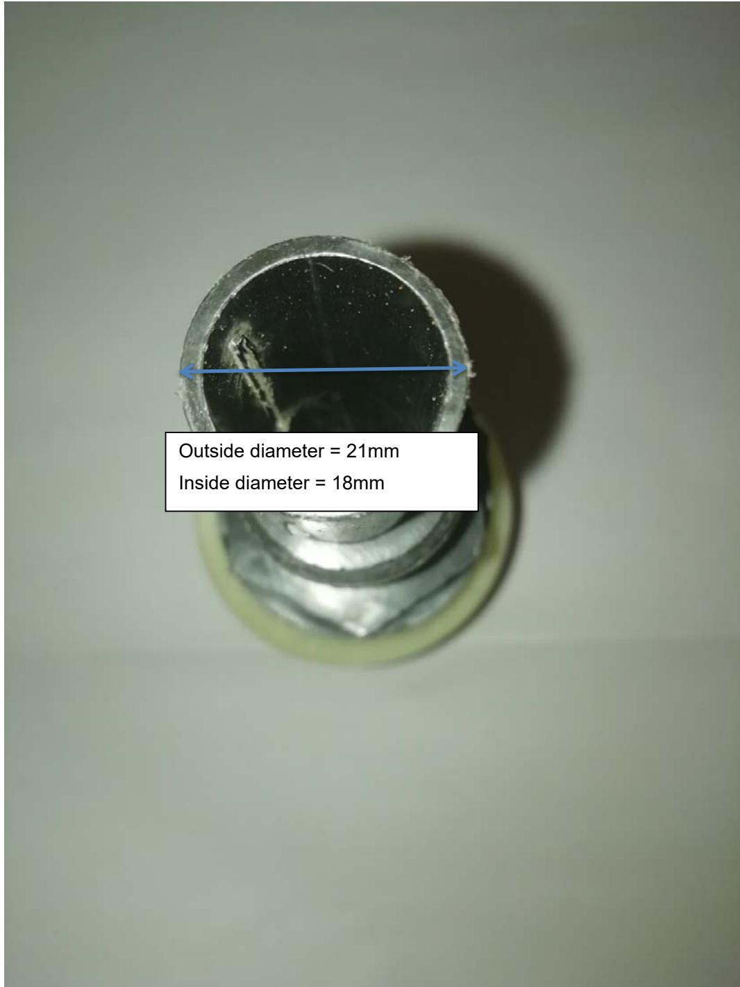
Figure 6: Bottom view of mixed bed nozzle
