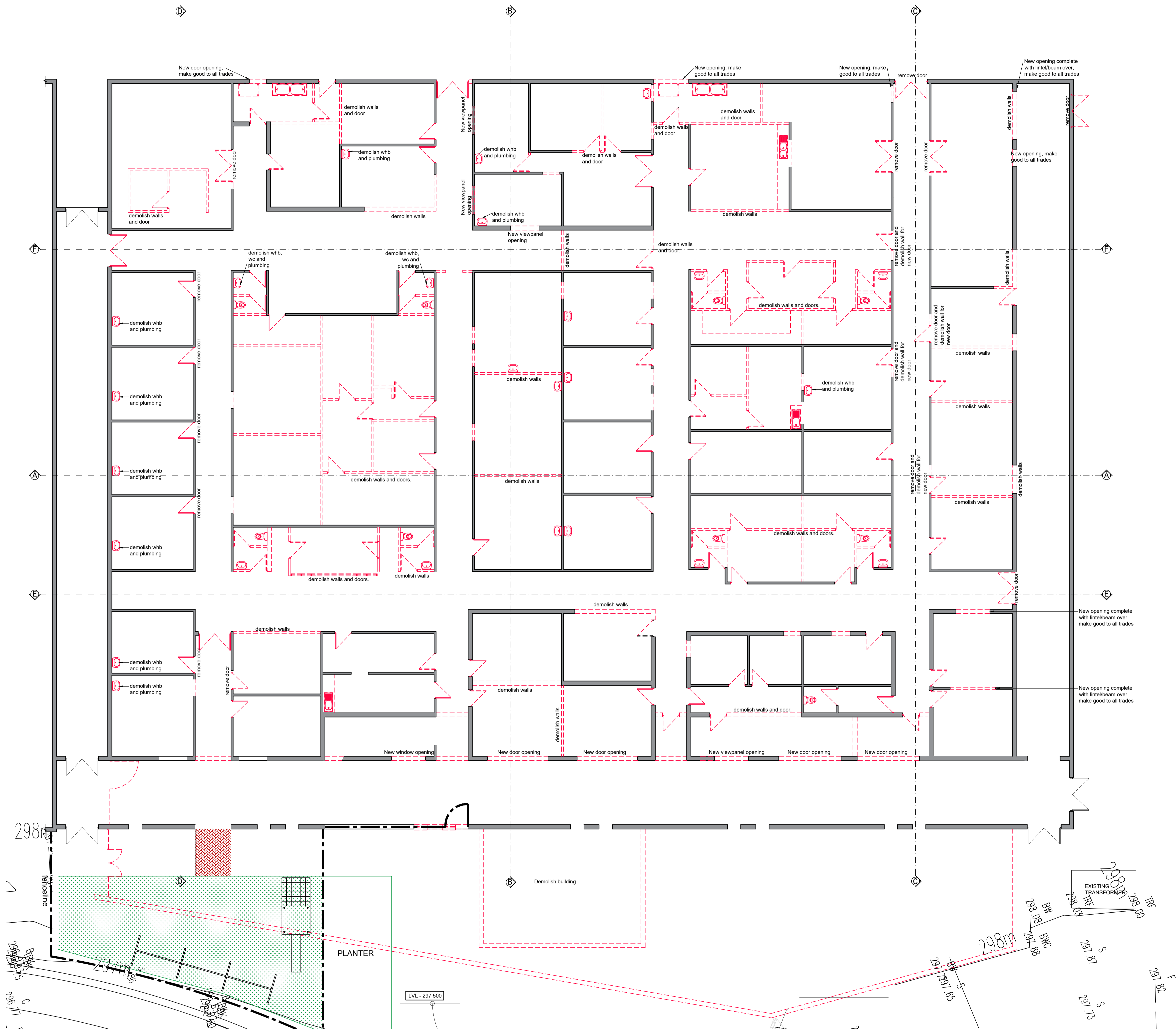
CP UNIT DEMOLITION PLAN SCALE 1:100
