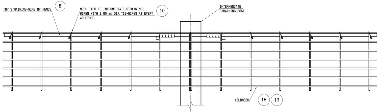
**WELDMESH ATTACHED TO TOP STRAINING WIRE**
