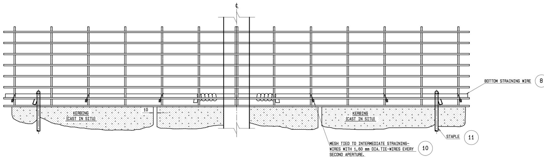
**WELDMESH ATTACHED TO BOTTOM STRAINING WIRE**
