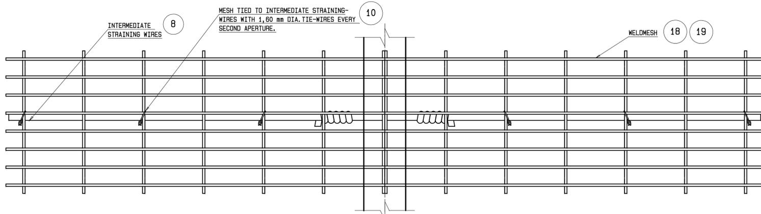
**WELDMESH ATTACHED TO INTERMEDIATE STRAINING WIRES**
