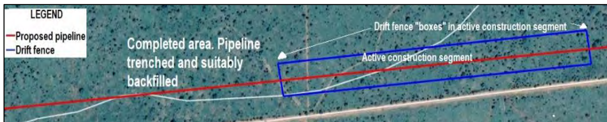
Figure 1: Example of how drift fences must encompass the active construction segment of the pipeline.
