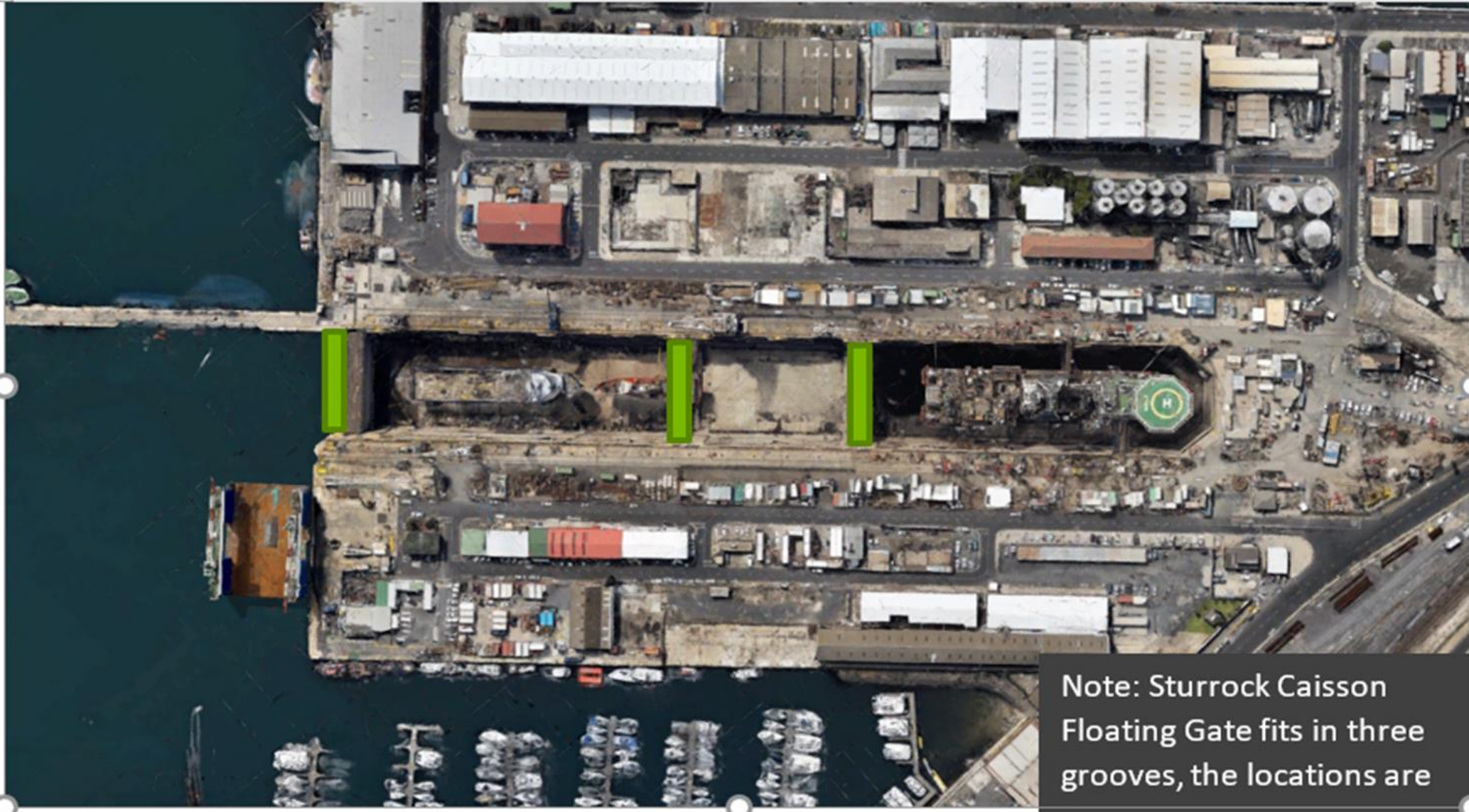
Figure 2: Plan View of Floating Gate Docking Grooves
