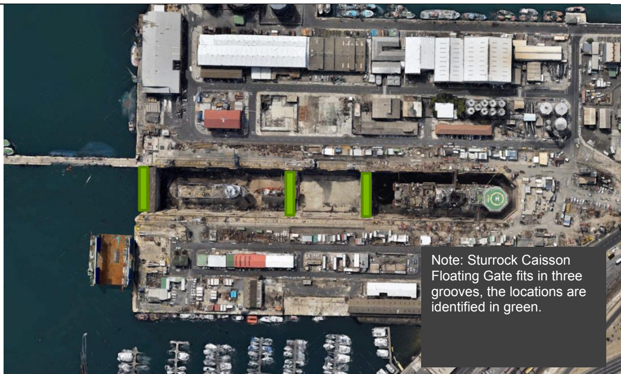
Figure 2: Plan View of Floating Gate Docking Grooves
