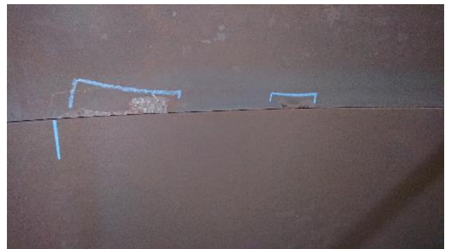
Figure 280: Exhaust – example of rubbing
