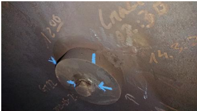
Figure 283: Exhaust – example of crack
