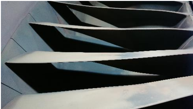
Figure 279: Turbine 4 th stage blades
