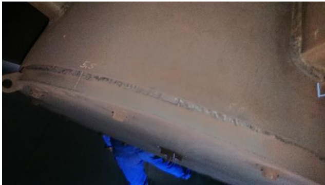
Figure 289: Exhaust – example of hammering
