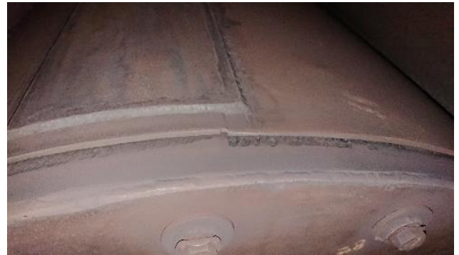
Figure 325: Exhaust – example of hammering
