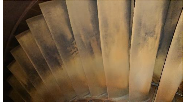
Figure 245: Turbine 4 th stage blades
