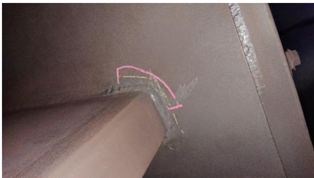
Figure 296: Exhaust – example of crack
