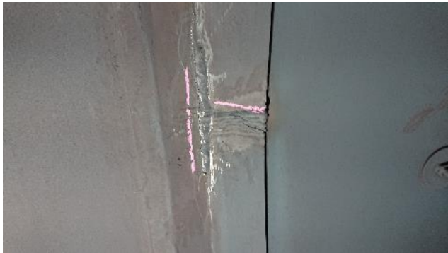
Figure 287: Exhaust – example of crack
