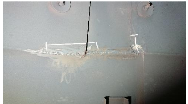
Figure 255: Exhaust – example of crack
