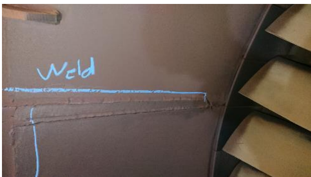
Figure 292: Exhaust – example of crack
