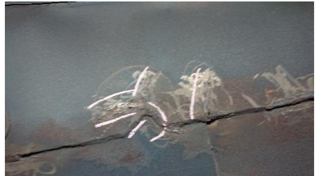
Figure 261: Exhaust – example of crack
