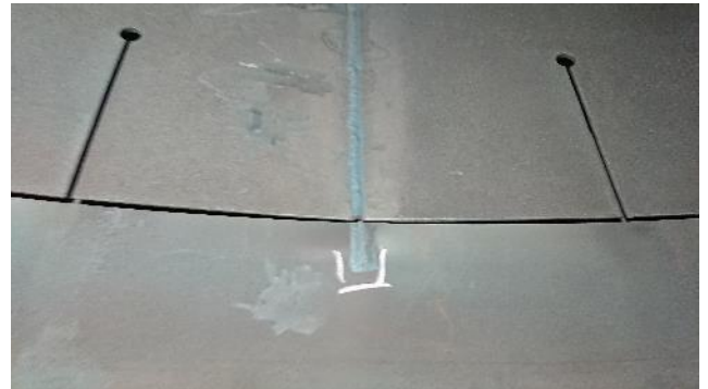
Figure 262: Exhaust – example of rubbing
