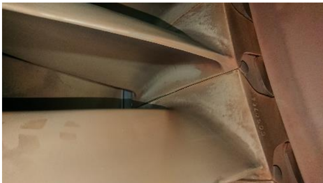
Figure 251: Turbine 4 th stage blades
