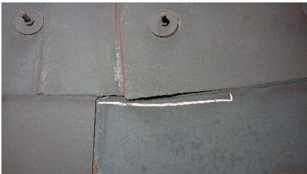
Figure 259: Exhaust – example of crack
