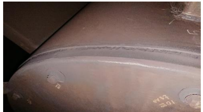
Figure 326: Exhaust – example of hammering
