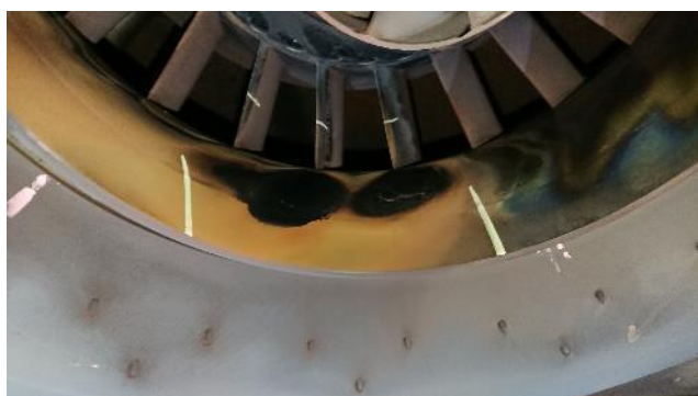
Figure 136: Burner 1-3
