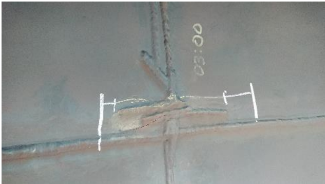
Figure 303: Exhaust – example of crack
