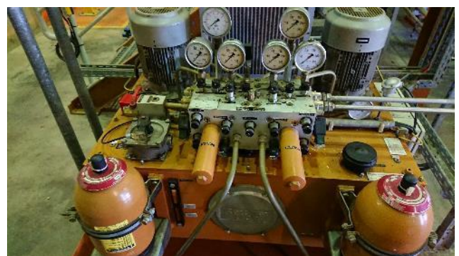
Figure 7: Control oil skid
