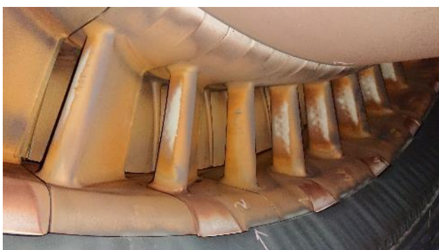
Figure 235: Turbine 1 st stage vanes & blades
