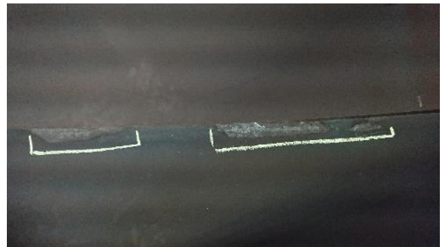
Figure 300: Exhaust – example of rubbing
