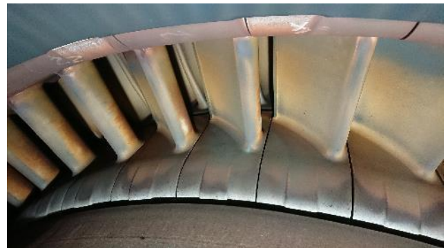
Figure 222: Turbine 1 st stage vanes & blades
