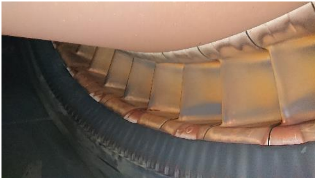
Figure 226: Turbine 1 st stage vanes
