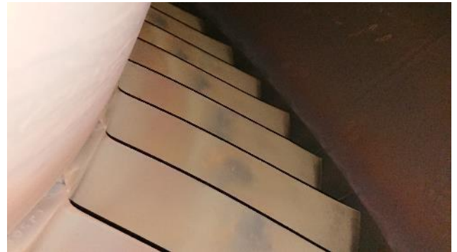
Figure 283: Turbine 4 th stage blades
