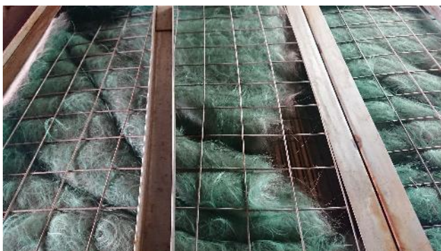
Figure 35: Coalescing filters
