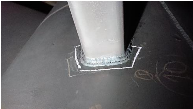
Figure 274: Exhaust – example of crack
