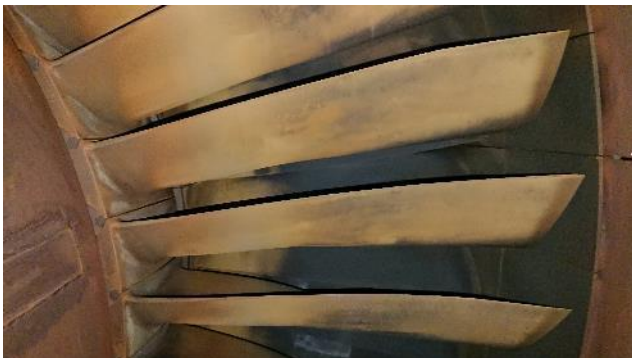
Figure 244: Turbine 4 th stage blades & vanes
