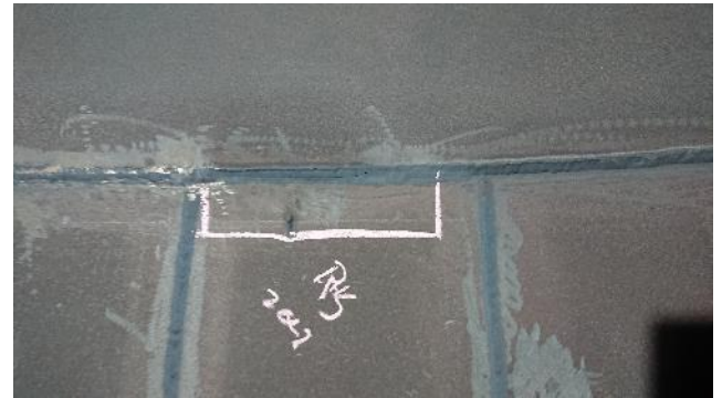
Figure 269: Exhaust – example of crack
