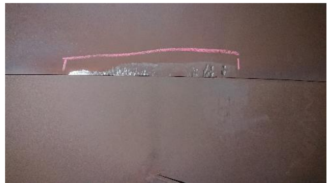
Figure 300: Exhaust – example of rubbing
