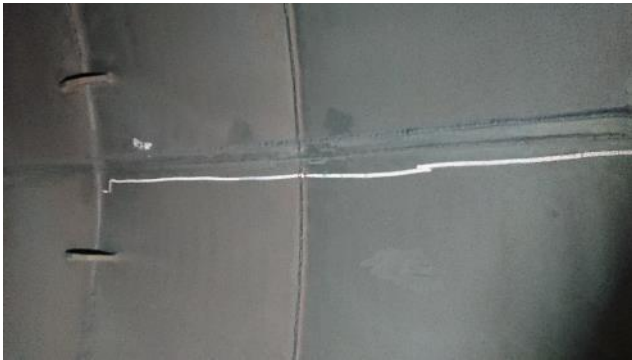
Figure 273: Exhaust – example of crack
