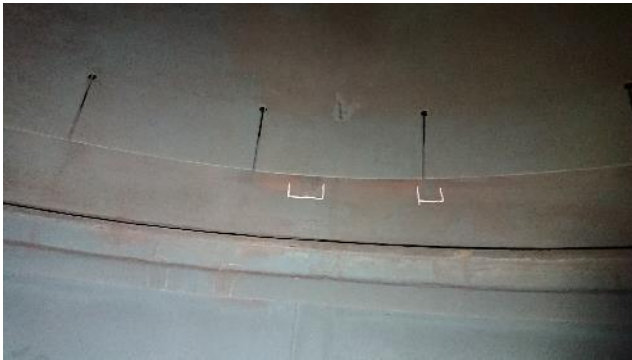
Figure 265: Exhaust – example of rubbing
