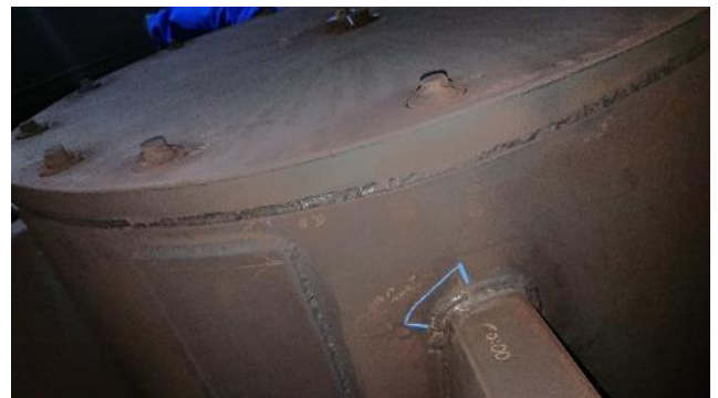
Figure 288: Exhaust – example of crack
