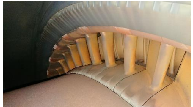
Figure 224: Turbine 1 st stage vanes & blades
