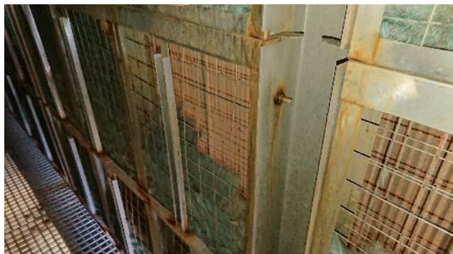
Figure 65: Coalescing filters
