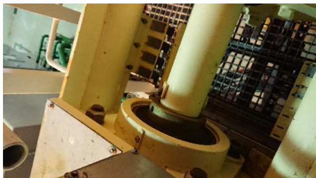
Figure 23: Compressor flap axel
