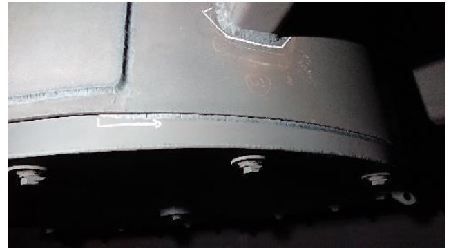
Figure 285: Exhaust – example of hammering
