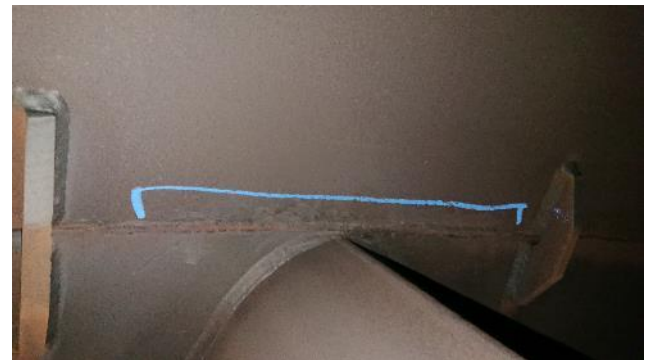
Figure 294: Exhaust – example of crack
