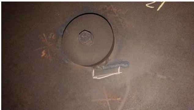
Figure 290: Exhaust – example of crack
