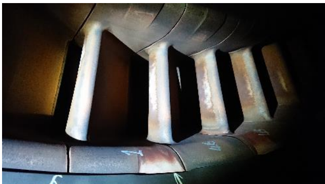
Figure 233: Turbine 1 st stage vanes & blades
