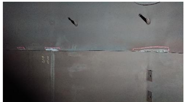
Figure 294: Exhaust – example of rubbing
