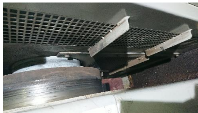
Figure 48: Exciter making shaft lift difficult
