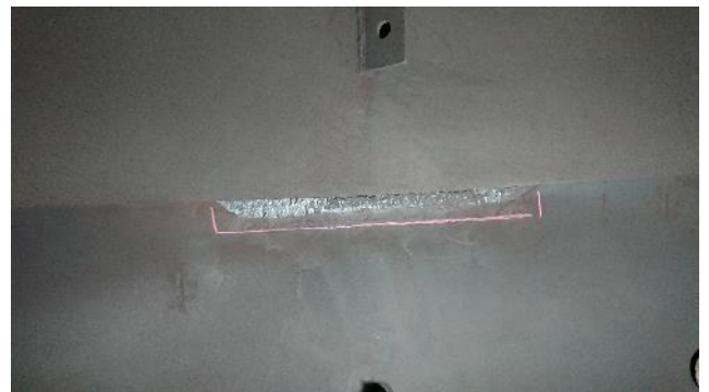
Figure 292: Exhaust – example of rubbing
