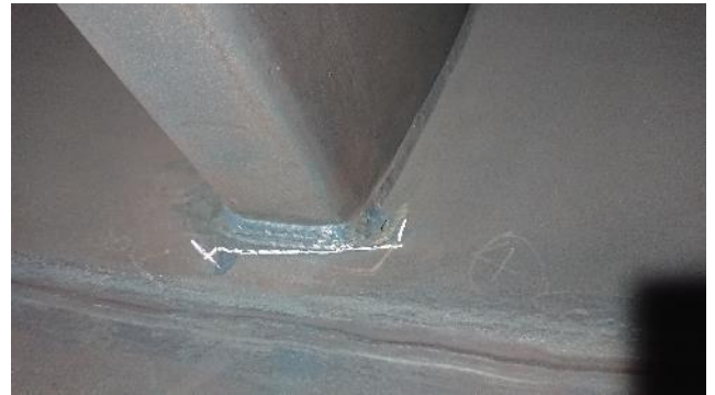
Figure 277: Exhaust – example of crack
