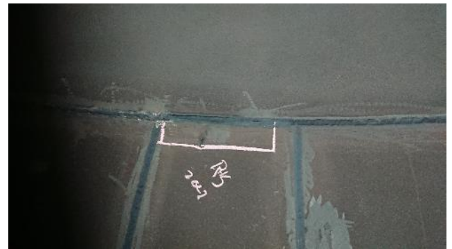
Figure 270: Exhaust – example of crack
