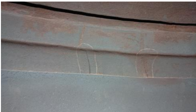
Figure 266: Exhaust – example of crack
