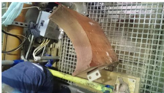
Figure 44: Tool used to raise shaft
