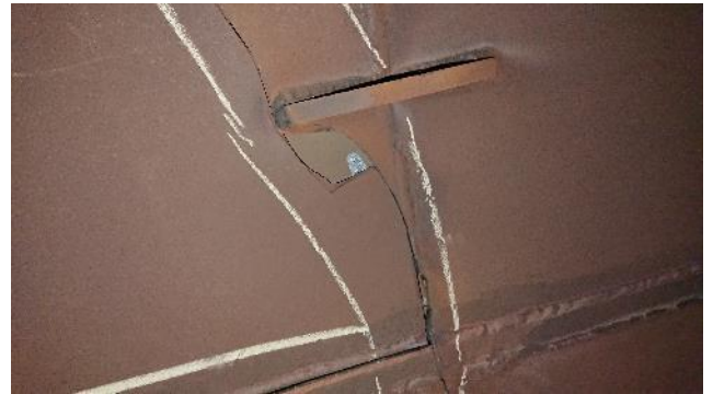
Figure 301: Exhaust – example of crack
