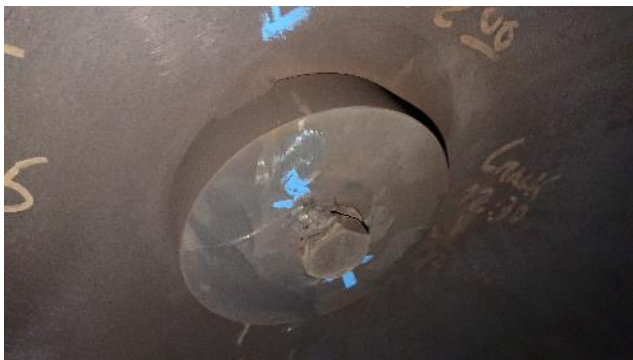
Figure 284: Exhaust – example of crack
