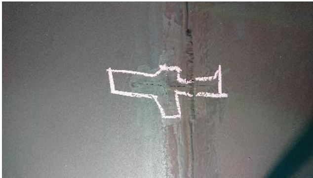
Figure 289: Exhaust – example of crack
