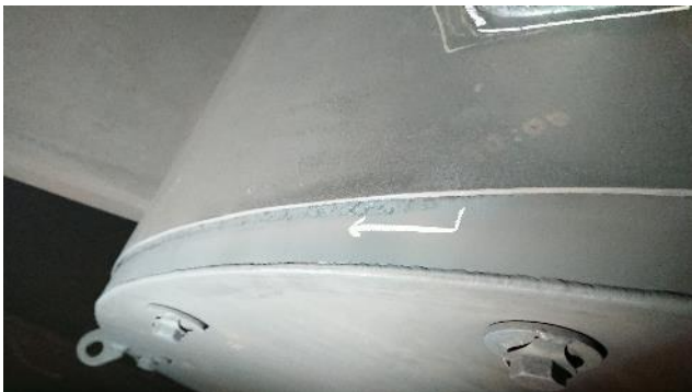
Figure 275: Exhaust – example of hammering
