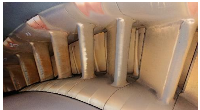
Figure 269: Turbine 1 st stage vanes & blades
