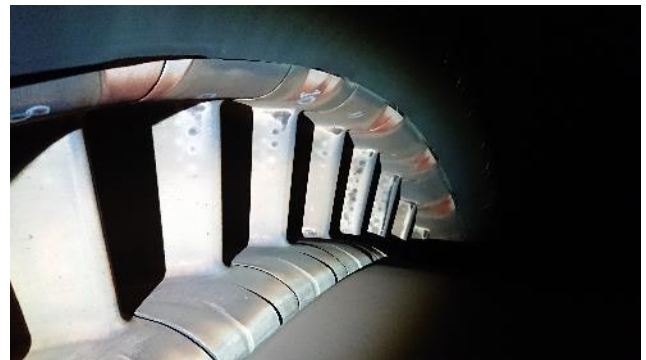
Figure 235: Turbine 1 st stage vanes
