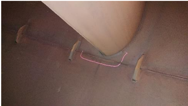
Figure 295: Exhaust – example of crack
