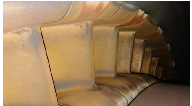
Figure 237: Turbine 1 st stage vanes
