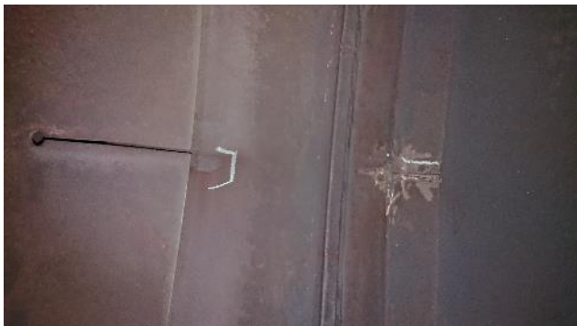
Figure 316: Exhaust – example of rubbing
