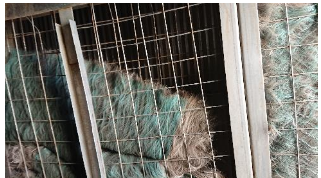
Figure 62: Coalescing filters
