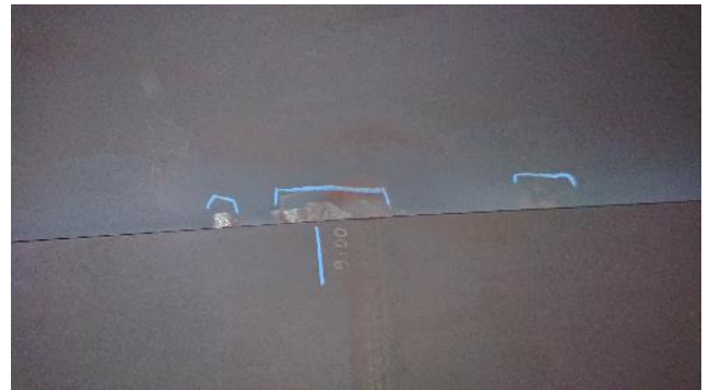
Figure 279: Exhaust – example of rubbing
