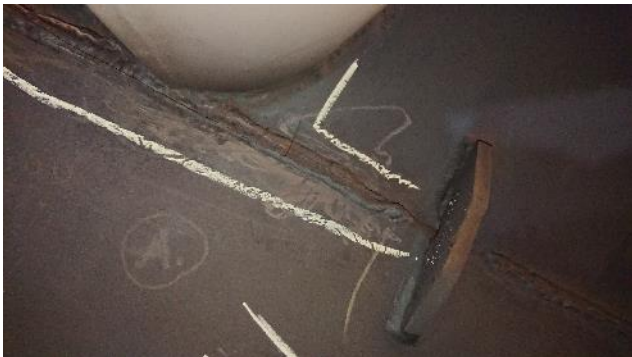
Figure 299: Exhaust – example of crack
