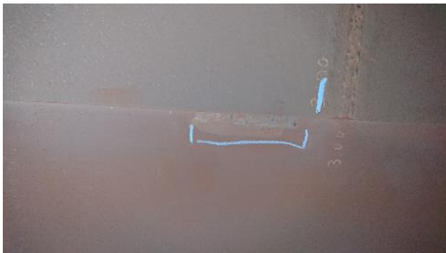
Figure 282: Exhaust – example of rubbing
