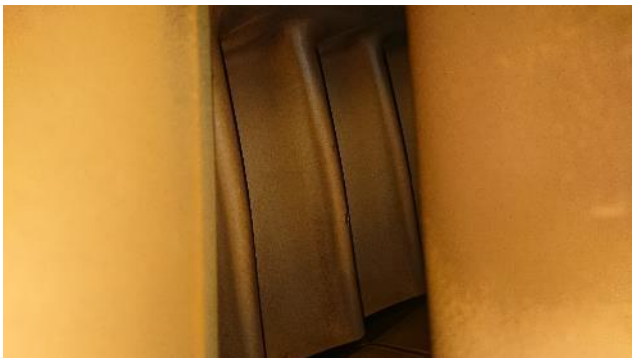
Figure 228: Turbine 1 st stage blades
