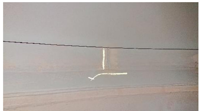
Figure 292: Exhaust – example of crack
