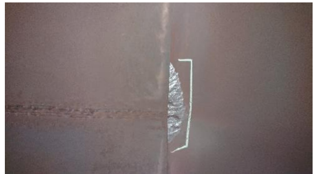
Figure 320: Exhaust – example of rubbing
