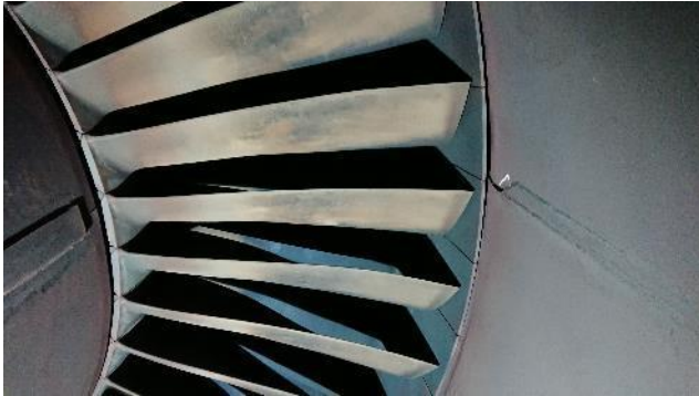
Figure 241: Turbine 4 th stage blades
