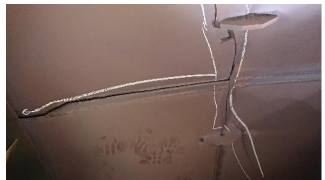
Figure 296: Exhaust – example of crack
