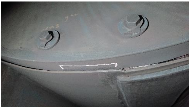
Figure 276: Exhaust – example of hammering
