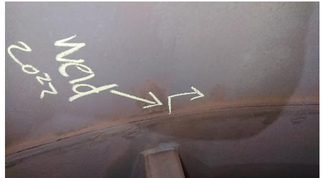
Figure 307: Exhaust – example of crack
