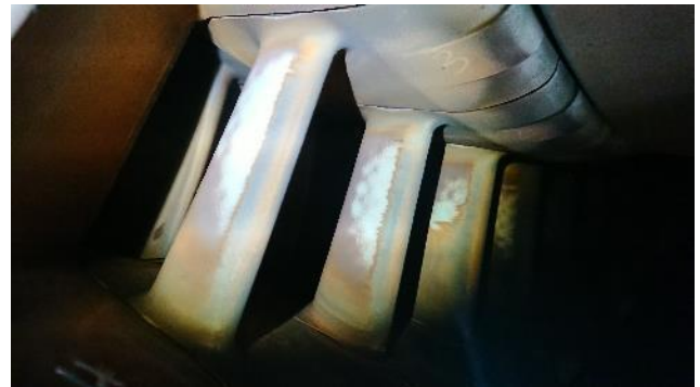
Figure 277: Turbine 1 st stage vanes
