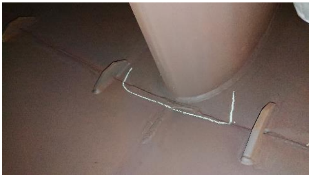
Figure 330: Exhaust – example of crack
