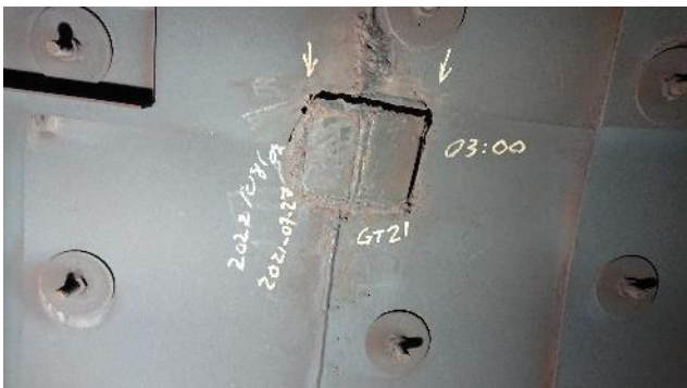
Figure 289: Exhaust – example of crack
