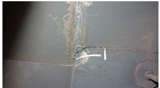
Figure 256: Exhaust – example of crack
