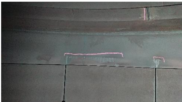
Figure 290: Exhaust – example of rubbing
