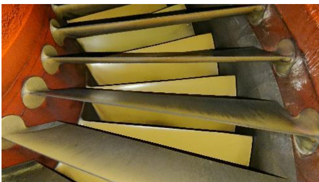
Figure 83: VIGVs & compressor 1 st stage blades
