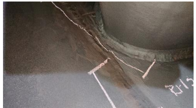
Figure 279: Exhaust – example of crack
