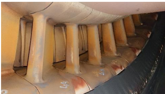
Figure 232: Turbine 1 st stage vanes & blades
