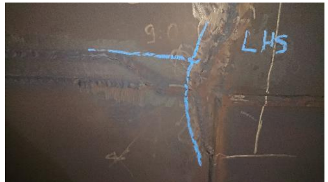
Figure 286: Exhaust – example of crack
