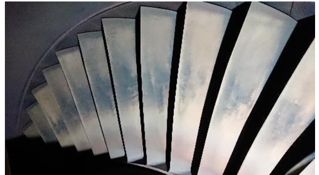
Figure 246: Turbine 4 th stage blades
