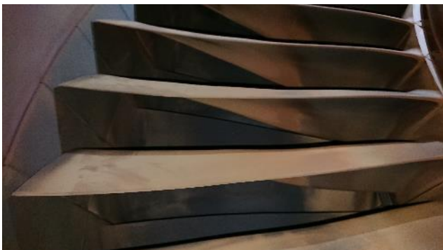
Figure 281: Turbine 4 th stage blades & vanes
