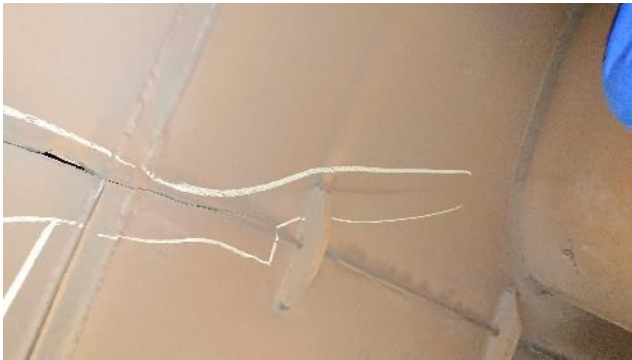
Figure 297: Exhaust – example of crack
