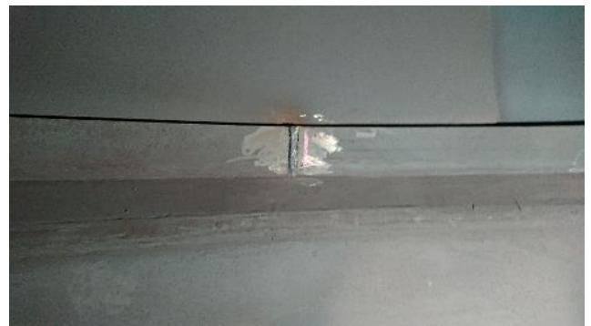
Figure 286: Exhaust – example of crack
