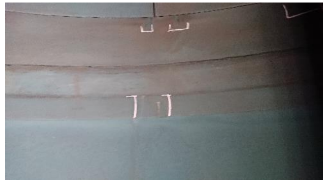
Figure 264: Exhaust – example of crack & rubbing
