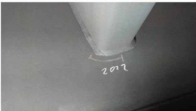
Figure 304: Exhaust – example of crack
