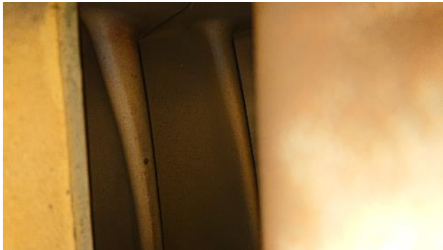
Figure 239: Turbine 1 st stage blades
