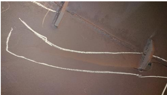
Figure 298: Exhaust – example of crack
