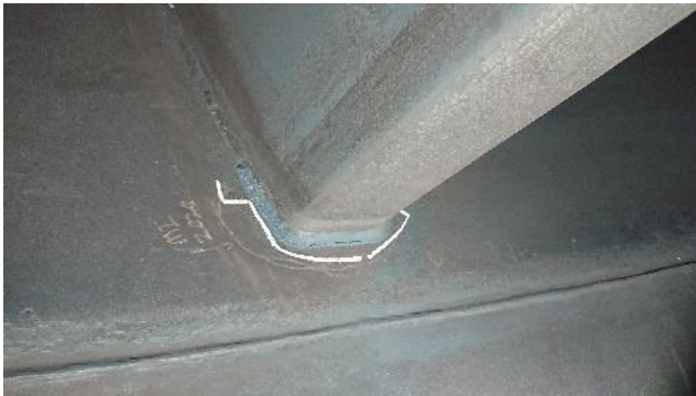
Figure 281: Exhaust – example of crack
