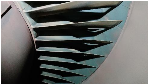
Figure 242: Turbine 4 th stage blades
