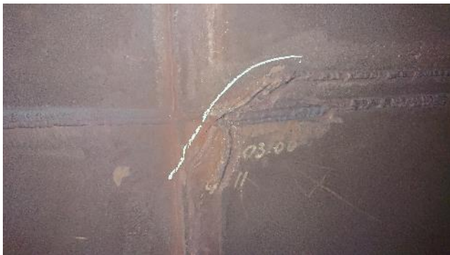
Figure 322: Exhaust – example of crack
