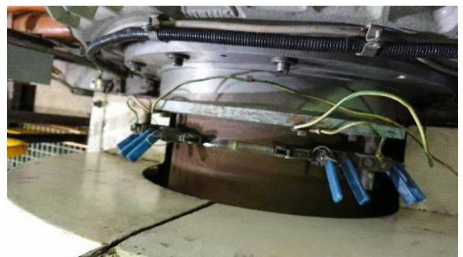
Figure 39: Generator TE bearing
