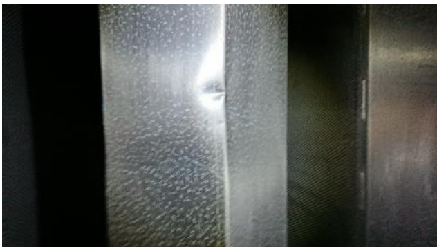
Figure 97: Dent on silencer
