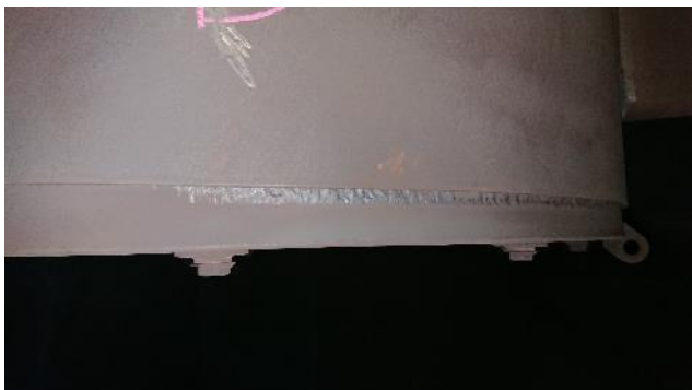
Figure 296: Exhaust – example of crack
