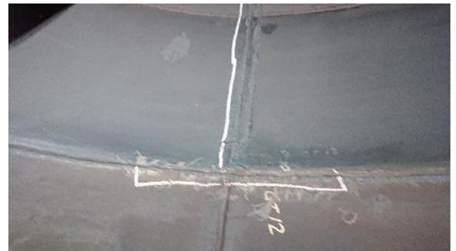
Figure 272: Exhaust – example of crack
