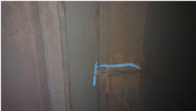
Figure 273: Exhaust – example of crack
