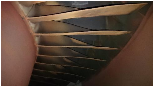
Figure 243: Turbine 4 th stage blades & vanes
