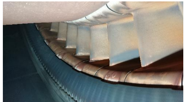
Figure 221: Turbine 1 st stage vanes
