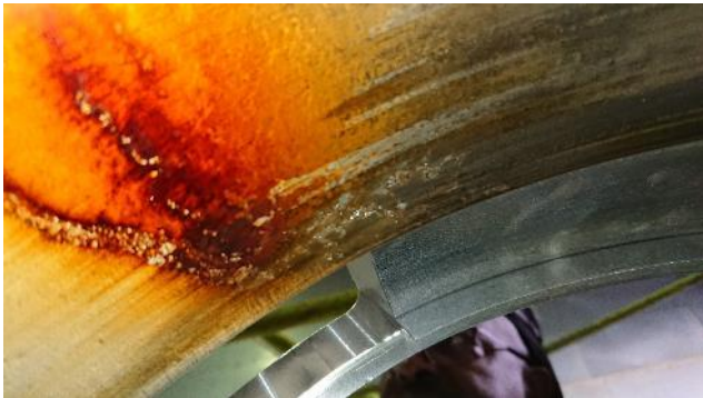
Figure 55: Generator bearing
