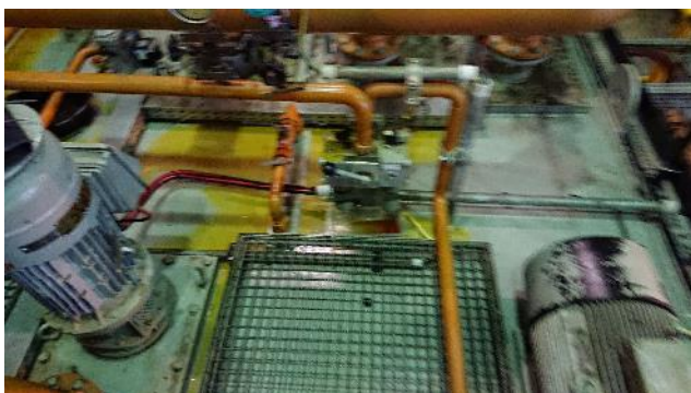
Figure 4: Lubricating oil skid
