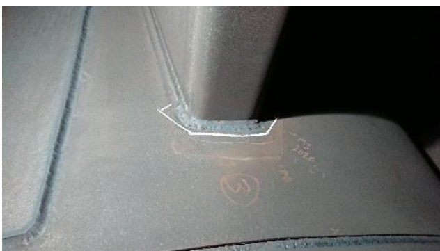
Figure 284: Exhaust – example of crack
