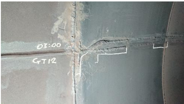
Figure 282: Exhaust – example of crack
