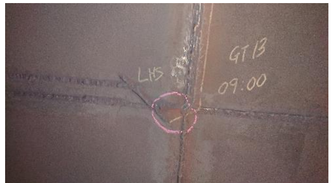
Figure 300: Exhaust – example of rubbing
