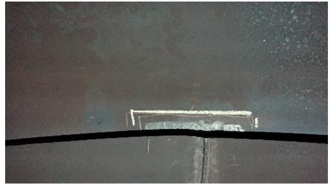
Figure 299: Exhaust – example of rubbing
