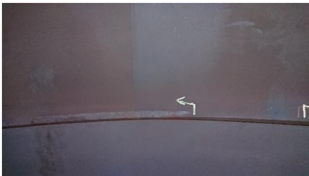
Figure 298: Exhaust – example of rubbing
