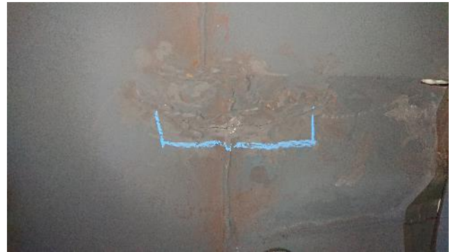
Figure 269: Exhaust – example of crack
