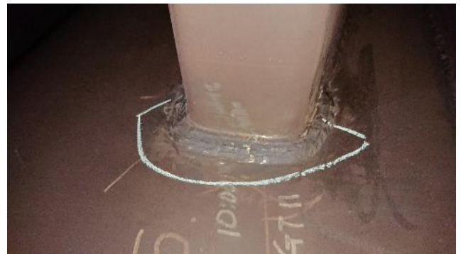
Figure 327: Exhaust – example of crack
