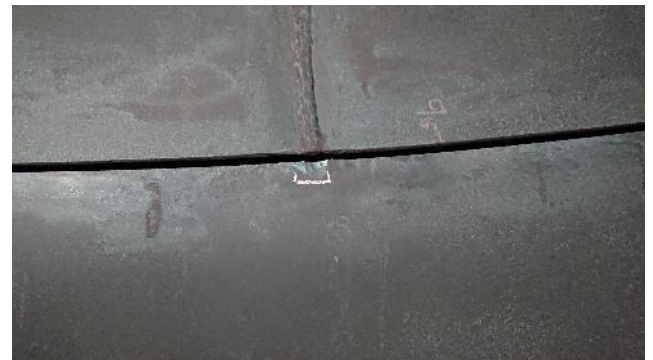
Figure 271: Exhaust – example of crack
