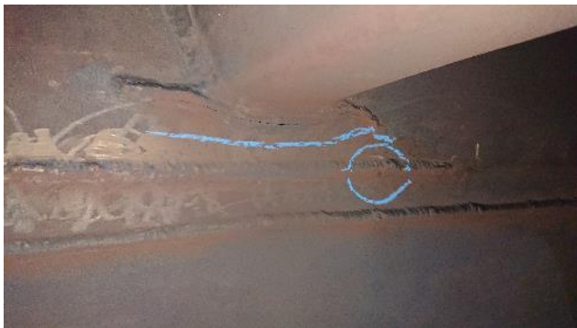
Figure 290: Exhaust – example of crack
