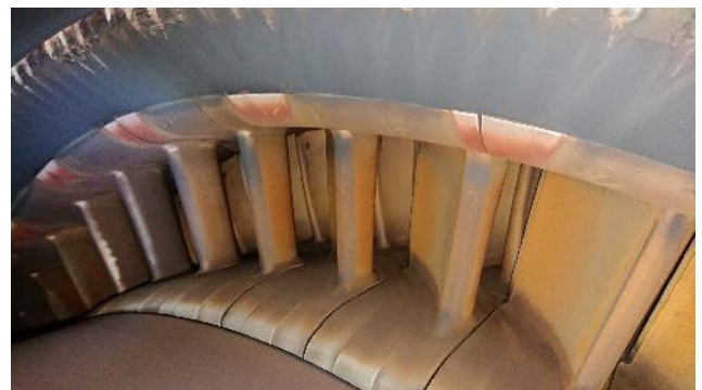
Figure 268: Turbine 1 st stage vanes & blades
