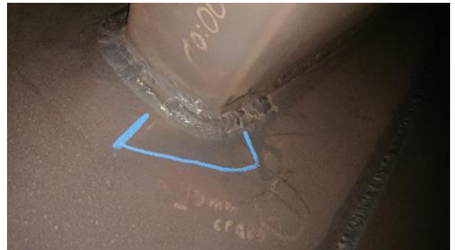
Figure 287: Exhaust – example of crack
