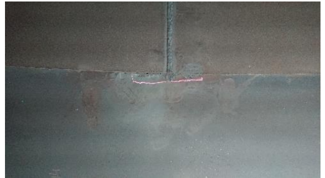
Figure 291: Exhaust – example of rubbing
