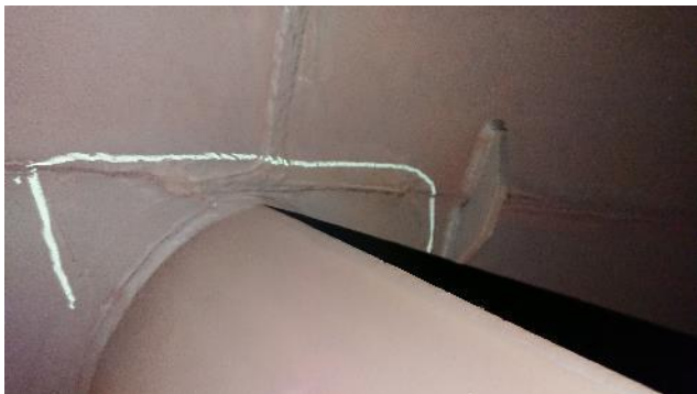
Figure 331: Exhaust – example of crack
