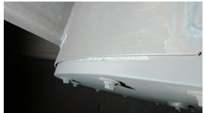
Figure 286: Exhaust – example of hammering
