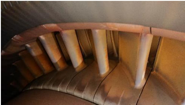
Figure 225: Turbine 1 st stage vanes & blades
