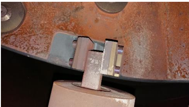
Figure 114: IC bottom key
