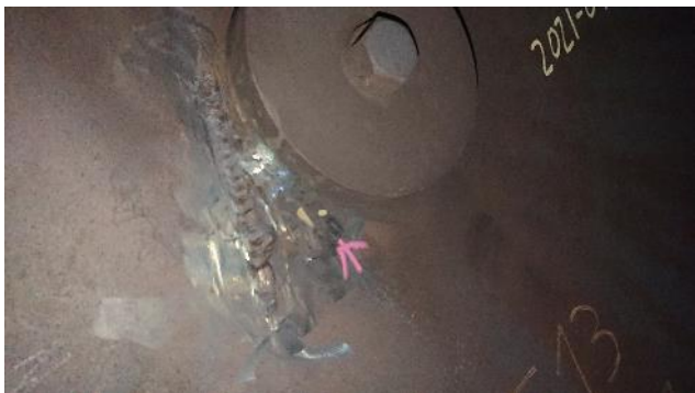
Figure 298: Exhaust – example of crack
