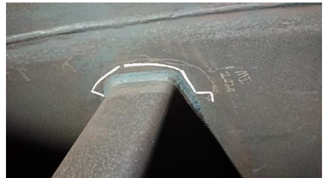
Figure 287: Exhaust – example of crack
