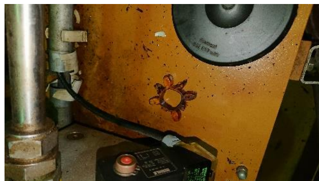
Figure 47: Old control oil pump coupling spacer
