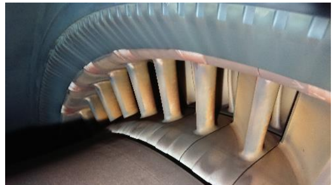
Figure 223: Turbine 1 st stage vanes & blades
