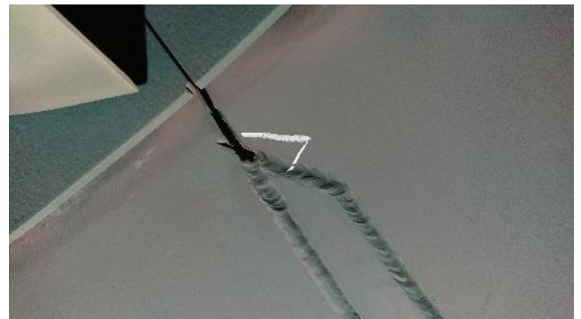
Figure 280: Exhaust – example of crack
