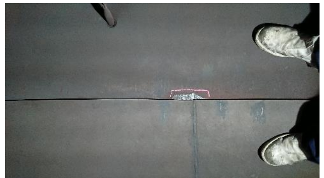
Figure 292: Exhaust – example of rubbing
