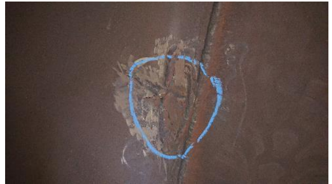
Figure 285: Exhaust – example of crack
