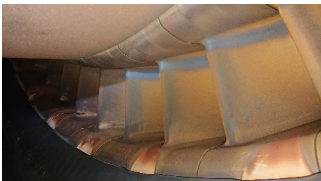
Figure 266: Turbine 1 st stage vanes
