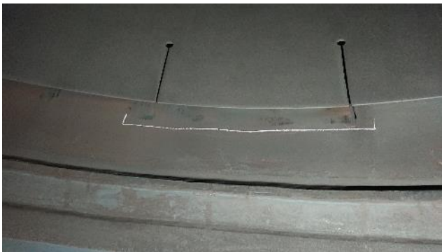
Figure 268: Exhaust – example of rubbing
