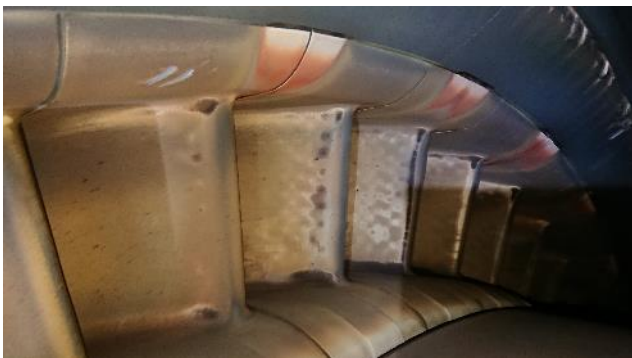
Figure 274: Turbine 1 st stage vanes
