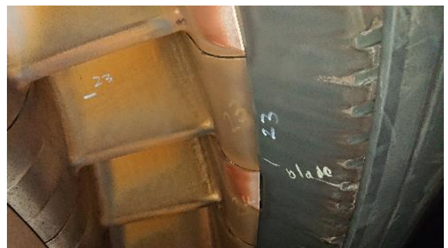
Figure 270: Turbine 1 st stage vanes
