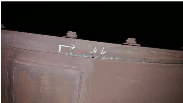
Figure 323: Exhaust – example of hammering
